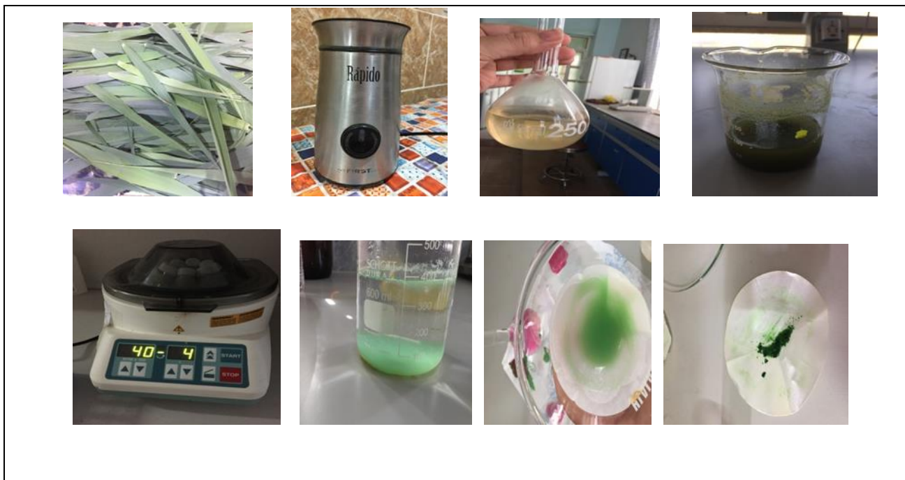
Figure (3.2): Steps of the preparation of Nickel (II) oxide nanoparticles using Arundo donax Leaves Extract.
